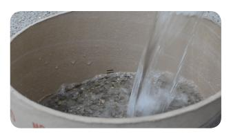
With all of our data points collected, we then perform the infiltration calculation using the mass of the water, the diameter of the infiltration ring and time of the test. With that information we have our final infiltration rate.
