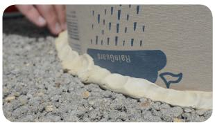
Once secure, prewet the concrete and infiltration ring with 8 pounds of water maintaining the head of water between the two marks on the interior of the ring. Begin timing as soon as the water hits the pervious concrete surface. When water is no longer present of the surface, record the elapsed time of the prewetting. The time elapsed determines the amount of water to be used in the actual test.
