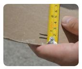
To install the infiltration ring, first clean the surface. The infiltration ring must meet certain size requirements and be marked with two lines on the interior to correctly perform the test. The ring is then placed on the cleaned surface and secured in place with plumber's putty.
